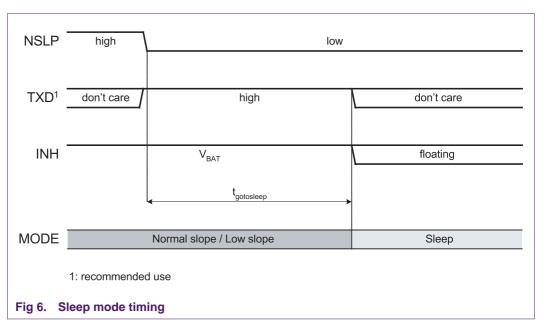
During Sleep mode, the internal slave termination resistor  $R_{SLAVE}$  between LIN and BAT is disabled; only a weak current source is present. This minimizes the current consumption in case LIN bus is short-circuited to ground.
