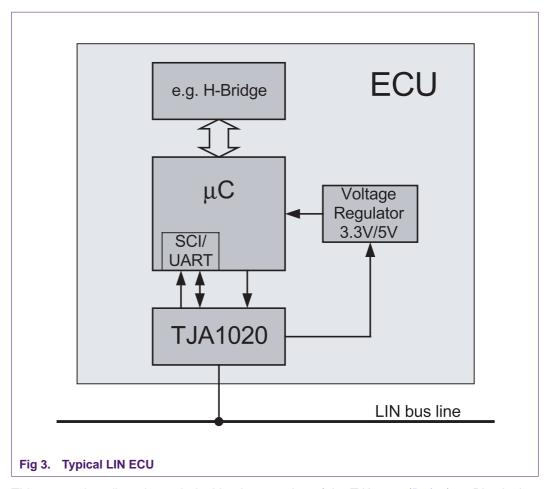
This report describes the technical implementation of the TJA1020 (Ref. 1) as Physical Medium Attachment within LIN. Its focus is to provide application hints / recommendations for the design of LIN electronic control units (ECUs) using the LIN transceiver TJA1020 from Philips Semiconductors (see Figure 3).
