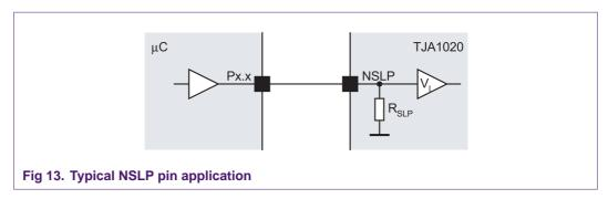
The minimum drive capability of the microcontroller port pin for the NSLP pin can be calculated with the following equation:
