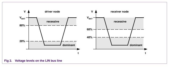
The LIN physical layer has been derived from the ISO 9141 (Ref. 3) standard but has some enhancements to meet the particular operation requirements in automotive environments such as EMC, ESD, etc. The LIN bus is a single-wire, wired AND bus with a 12 V-battery related recessive level. The voltage levels on the LIN bus line are shown in Figure 2.
