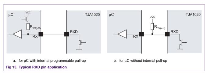
The minimum pull-up resistor  $R_{RX,min}$  is defined by the drive capability of the TJA1020's RXD output pin. The maximum pull-up resistor  $R_{RX,max}$  depends on the maximum delay of the rising edge  $t_{rPropRX}$  caused by the RC-load on RXD:
