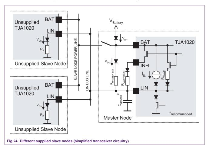
The maximum master termination resistor  $R_{\text{MASTER-BAT}}$  can be calculated with the following equation:
