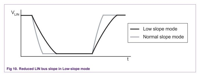
The Low-slope mode is entered by a low level on the TXD pin in conjunction with a high level on the NSLP pin maintained for at least  $t_{gotonorm,max}$  (Ref. 1). The mode transition is executed when  $t_{gotonorm}$  (Ref. 1) is expired. The timing of a transition from Sleep or Standby mode to Low-slope mode is shown in Figure 11.
