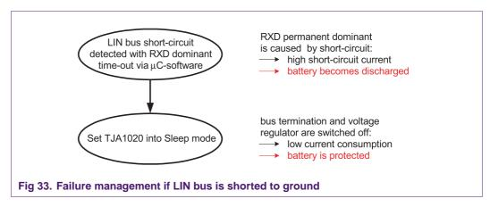
Once the LIN bus is shorted to ground this can be detected in software monitoring the continuous dominant level on RXD.
